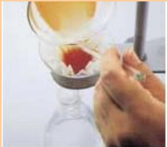
Filtration using a folded filter paper in an analytical funnel
